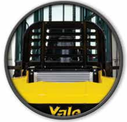
Hinged hood gives access to radiator cooler
